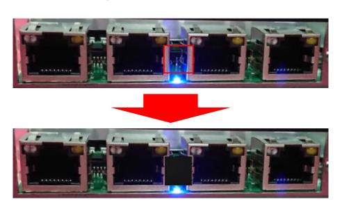
1. Insert the CMI module vertically into the female connector on system's mainboard until it's connected firmly and fasten 4 copper pillars to fix it.
