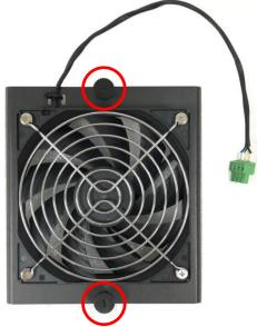
2. Slide the FAN into the middle groove of chassis as illustrated. Tighten the 2 screws to fix it onto chassis.
