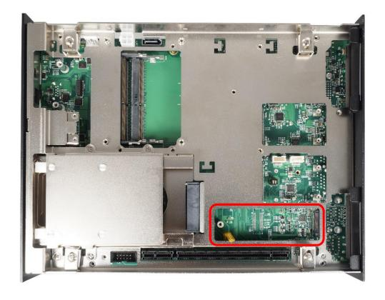
3. Tilt the Mini-PCIe module at a 45 degree angle and insert it to the slot until the gold-pated connector of module contacted firmly with the slot.
