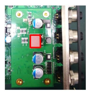
6. Please paste the heatsink onto the CFM-PoE module carefully.
