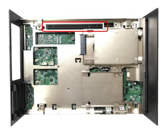
7. Install the module assembled in step 4 into the riser card slot, and fasten the 4 screws to secure it.
