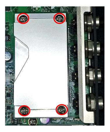
6. Please paste the thermal pad onto the heatsink carefully.
