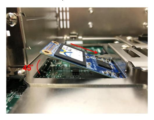
3. Press down the module and use previous two screws to fix the module.
