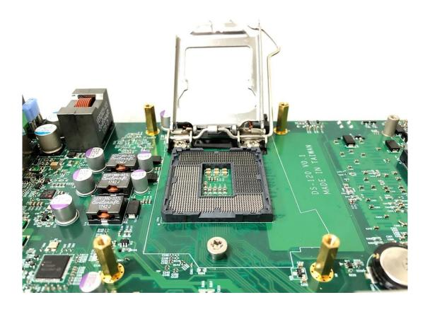
3. Align the notches on CPU with the alignment post on socket.
