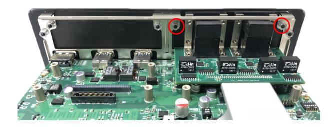
5. Fasten the 8 D-Sub jack screws as marked on photo.
