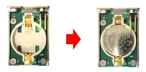
4. Insert the battery bracket firmly and fasten the screw.
