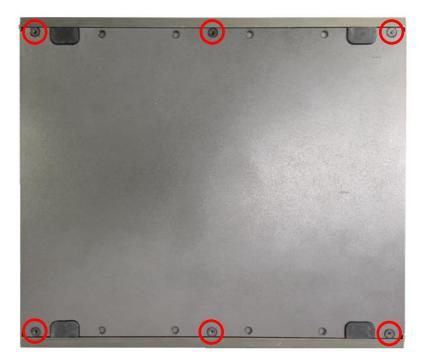
2. Remove the bottom cover from the chassis.
