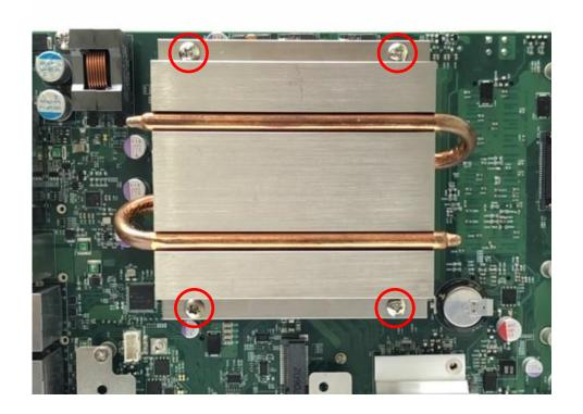
7. Place thermal pad on the top of CPU heatsink in order to provide a seamless contact with the body of chassis to create a efficient heat dissipation.
