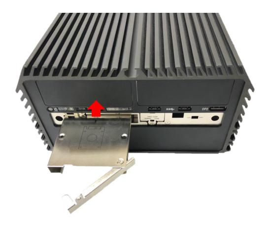
6. Place the rotating arm back and fasten the screw.
