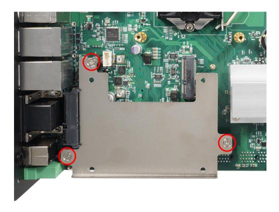
2. Make the PCB side of the HDD face up, place the HDD bracket on it. Ensure the direction of bracket is correct and use 4 provided screws to assemble HDD and HDD bracket together.
