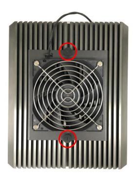
4. Connect the FAN cable to external fan power connector at rear panel.
