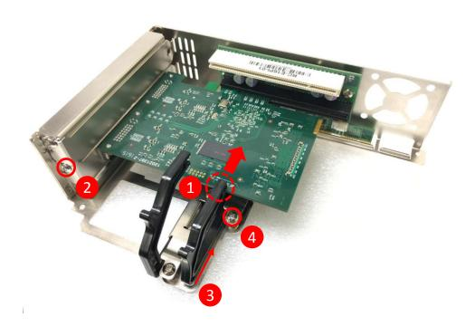
6. Locate the riser card slot on bottom side of system.
