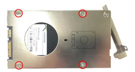
5. Align the HDD bracket with the entrance of HDD bay. Holding the rotating arm and insert the HDD bracket until the connector of HDD contact the SATA connector firmly.
