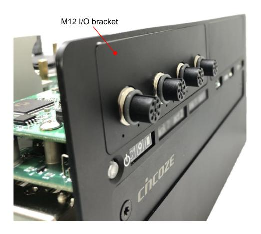
5. Fasten 2 hex nuts from the back side of the bracket.
