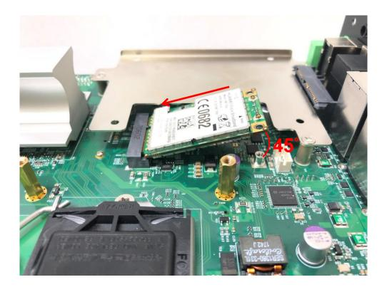
4. Press down the module and fasten two screws to secure the module.
