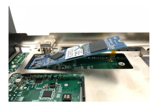
4. Press down the module and use previous one screw to fix the module.
