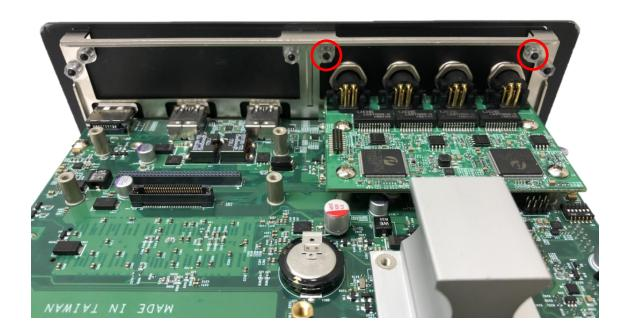
6. Fasten the 4 ring nuts onto M12 jacks.
