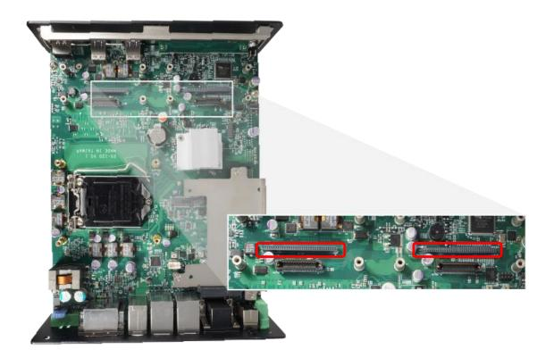
3. Insert the CMI module carefully into the CMI connector on main board. Fix it with 2 screws.
