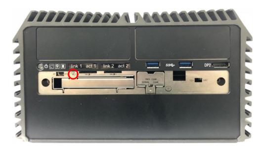
3. Move the rotating arm out and pull the HDD bracket out.
