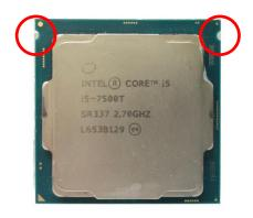
4. The notches of socket provide the space for fingers while lowering the CPU, hold the CPU by the edges toward the notches and insert the CPU gently.
