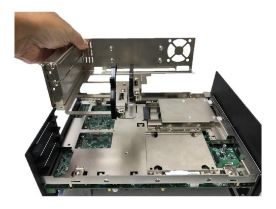
3. Assemble the riser card with extension bracket together and fasten with the 4 screws.
