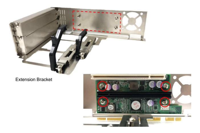
4. (1) Loosen the screw to remove I/O bracket. (2) Loosen the 2 screws halfway to allow the card retainer to be adjustable.
