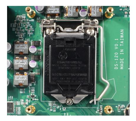
2. Press the CPU socket lever and pull it aside away from the socket to unlock it. Pull back the lever to open the socket.
