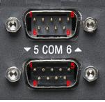
Note: COM3/4/5/6 are isolated COM, each pin5 (GND) is independent.
