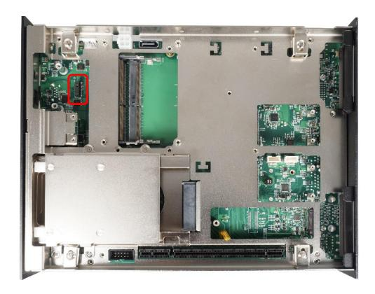
2. Insert the power ignition module carefully into the connector on main board. Fasten 2 screws to fix it.
