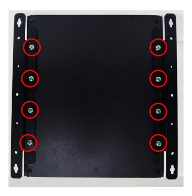
2. Fasten the screws through the bracket mounting hole to mount system on the wall.
