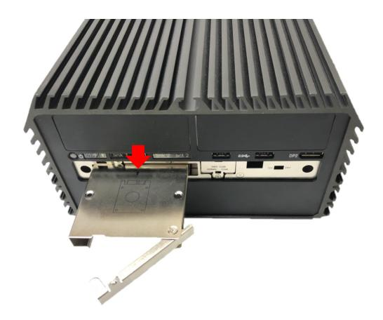
4. Make the PCB side of the HDD face up, place the HDD bracket into it. Ensure the direction of bracket is correct and use 4 provided screws to assemble HDD and HDD bracket together.
