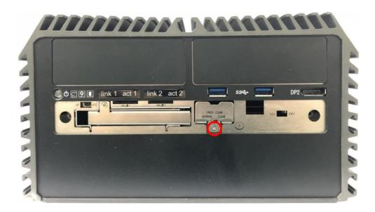
2. Pull out the CMOS battery bracket with assistance of a tweezer.
