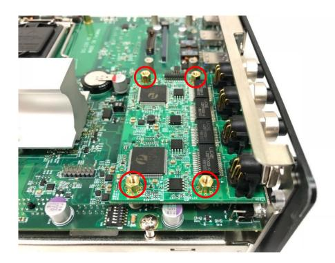
2. Insert the CFM-PoE module vertically into the female connector on CMI module until it's connected firmly.
