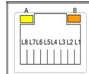
LAN1 to LAN8 (RJ45 type with PoE) are based on the Intel i211 with PoE support on the rear side panel.
