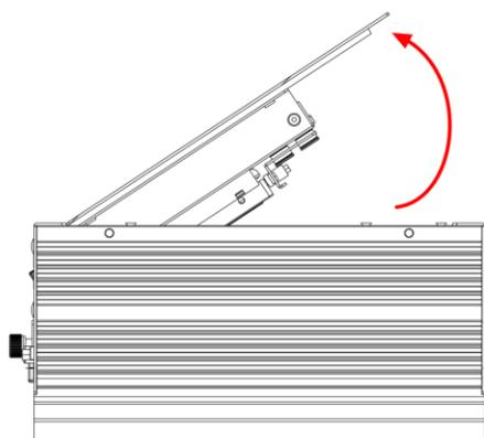
※ After lifting up the cover, please remove the fixed SATA cable first and then put the cover aside.
