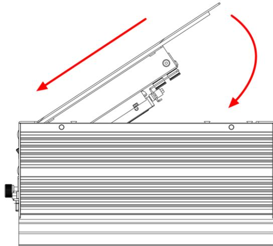
**Step 9 Slide the SATA trays back and fasten screws firmly to complete the installation.**
