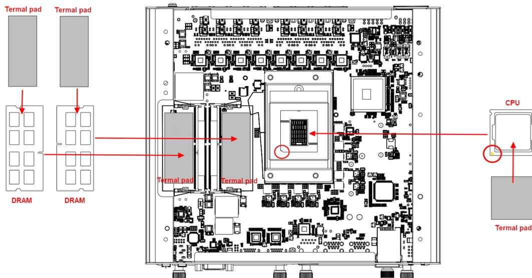
※ The memory module is locked by two latches on the sides. We recommend using "LDC737" silicone on both sides of the memory for optimal protection against vibration.
