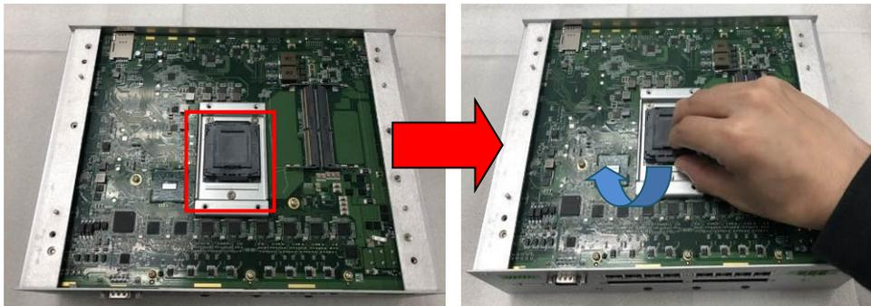
**Step 5 Stick thermal pad and install DRAM and CPU.**
