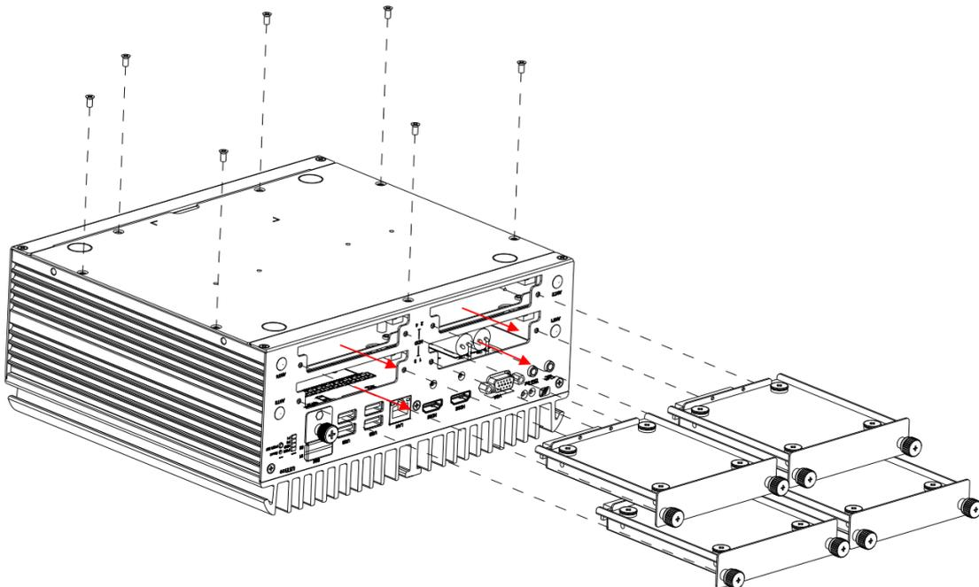
**Step 4 Loosen all screws and open the bottom cover carefully.**
