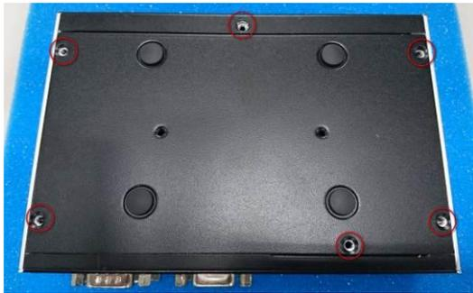
**Step 2** Remove 4x rubber pad as shown.
