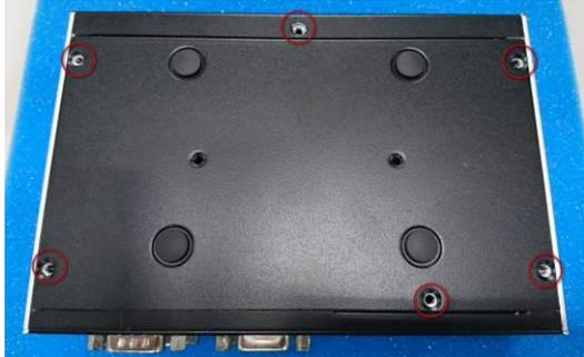
**Step 2** Install the module card and fasten screw as shown.
