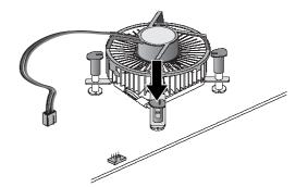
3. Make sure the CPU fan is plugged to the CPU fan connector.
