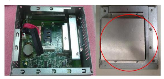
**Step 4** Loosen these screws and remove the Hard Disk Drive bracket.
