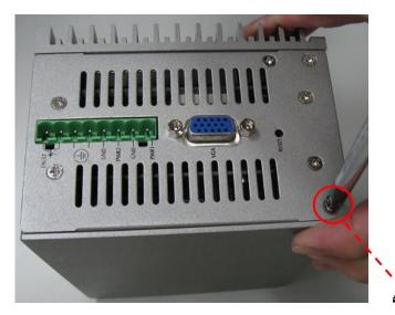
Step 3 Loosen these screws and remove the Thermal & CompactFlash TM fixing bracket from the system
