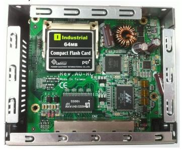
**Step 6** Put the Thermal & CompactFlash TM fixing bracket back to the system, and fasten screws tight close the Thermal & CompactFlash TM fixing bracket..
