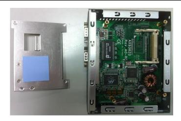
Step 5 Insert the CompactFlash<sup>TM</sup> card into the socket until it is firmly seated.
