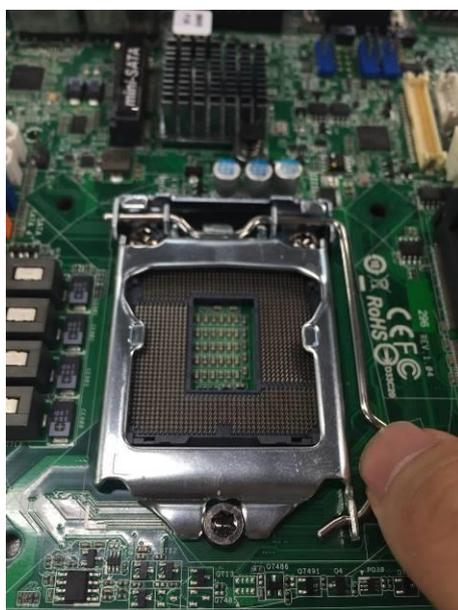
**Step 3** CPU aims at the socket and places the package carefully into the socket by purely vertical motion.
