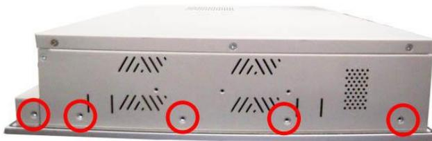
**Step 2** Fixing the rack-mount bracket to the left and right of the system.
