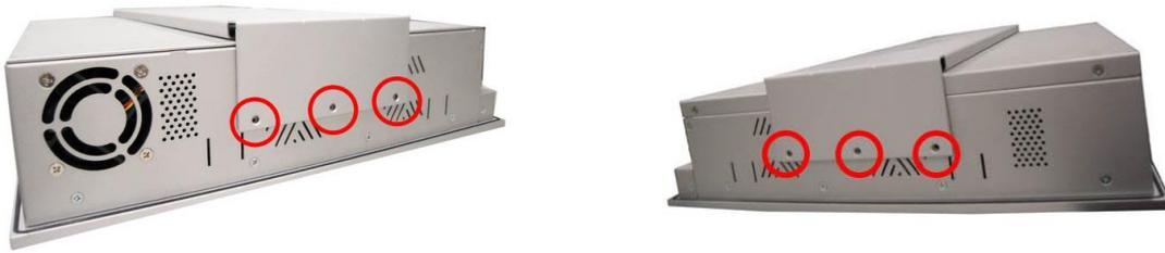
▲ Fixing the bracket by six screws on the left and right side.
