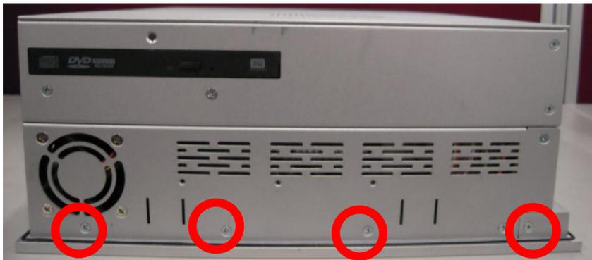
**Step 2** Fixing the rack-mount bracket to the left and right of the system.
