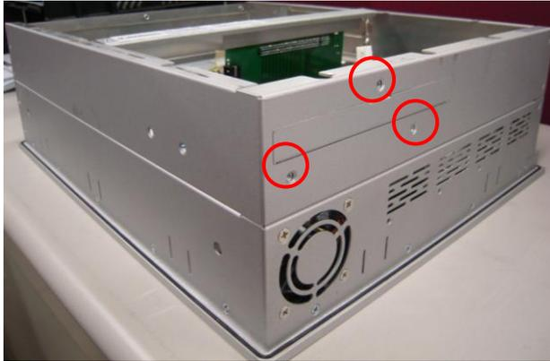
**Step 3** Fixing the optical drive on the bracket.
