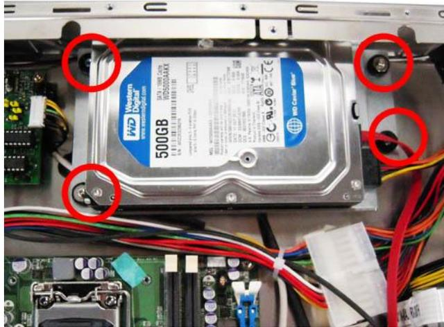
**Step 5** Plug the power and SATA cables to connectors. Installation completes.
