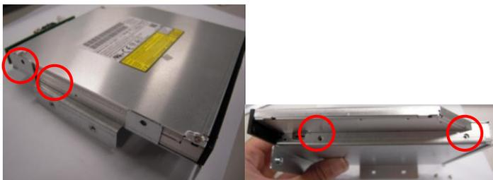
▲ Fixing optical drive by 4 screws.
