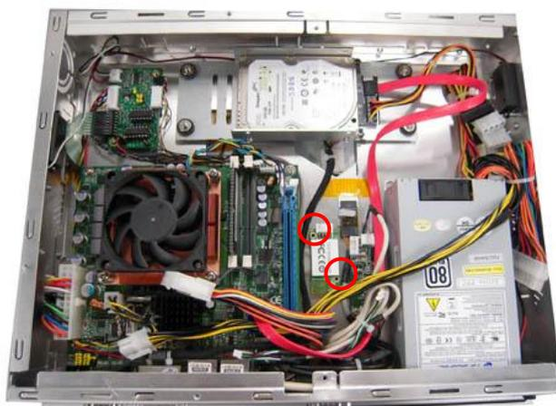
**Step 3** Plug in USB cable to the connector of WIFI module. And, find the built-in Antenna cable and connect it wireless LAN card.
