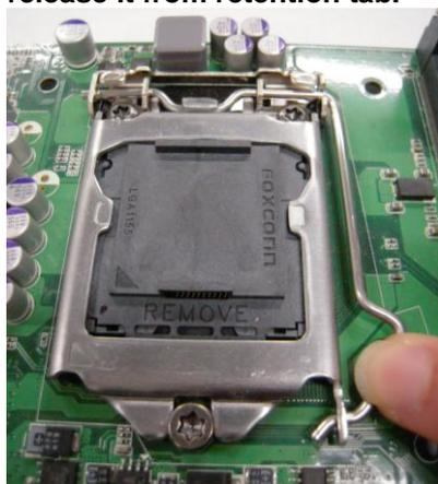
**Step 2** Lift the tail of the load lever and rotate the load plate to fully open position. And, remove the protective plastic cover.
