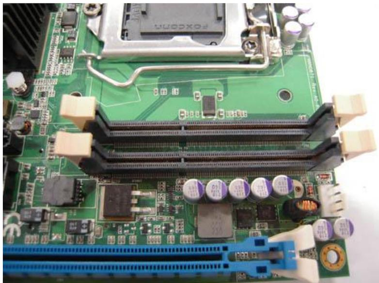
**Step 2** Push the latches on each side of the SO-DIMM slot down.
