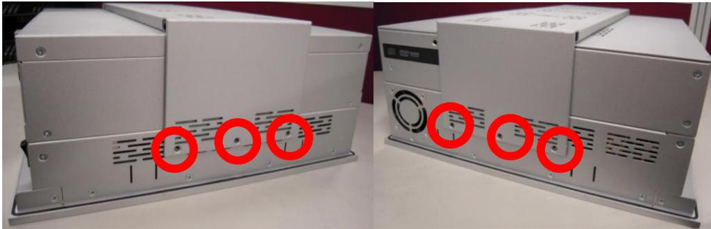
▲ Fixing the bracket by six screws on the left and right side.
