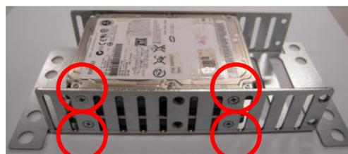
▲ Fix the 2.5" HDD on the right and left side bracket
