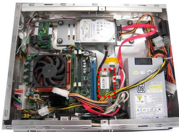
**Step 2** Fixing the wireless LAN module by 2 screws.
