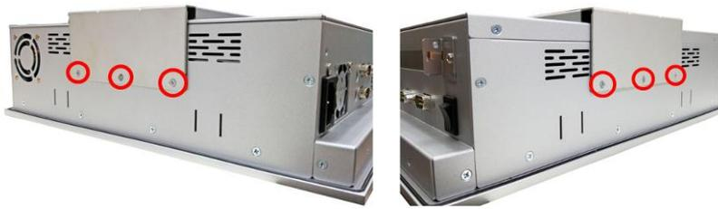
▲ Fixing the bracket by six screws on the left and right side.
