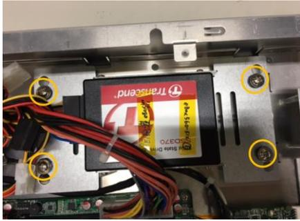
**Step 3** Fix the HDD on bracket by the screws.
