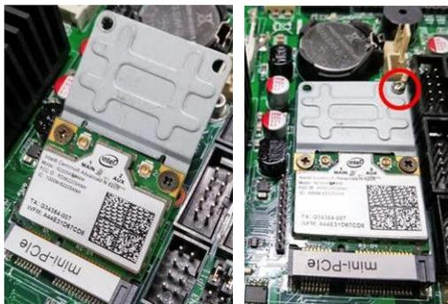
**Step 3 Find the built-in Antenna cable and connect it wireless LAN card.**
