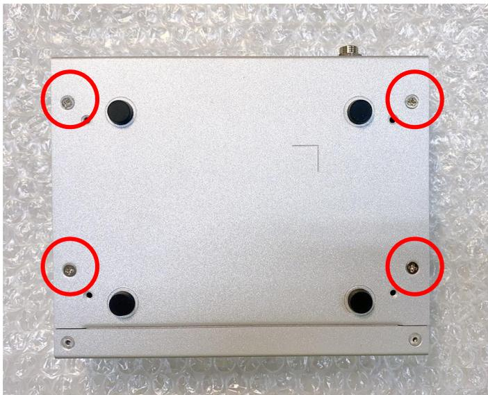
**Step.3** Identify the full-size mini PCIe slots, insert a mini PCIe module into the sockets and then fasten all screws.
