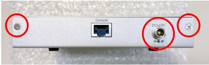
**Step.2** Loosen four screws to remove bottom cover.
