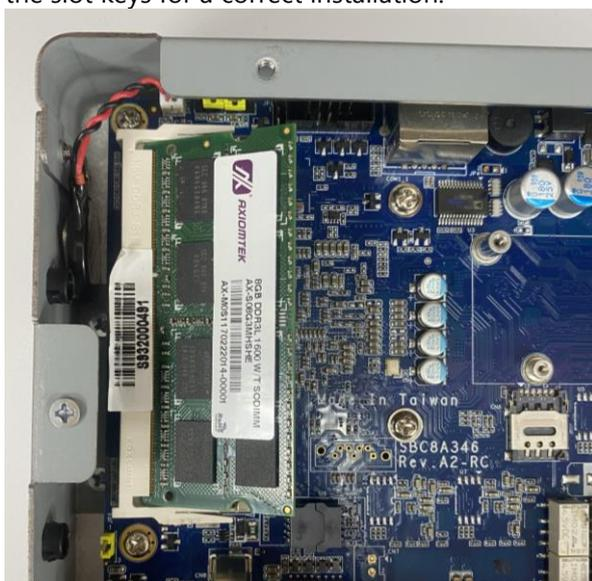
3. Install the memory module into the slot and push it firmly down until it is fully seated. The slot latches are levered upwards and clipped onto the edges of the DIMM.
