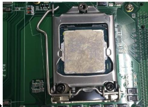
**Step 5** Apply thermal grease on top of the CPU
