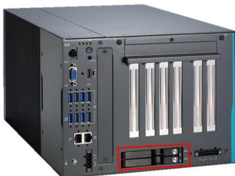
**Step 2** Align the connector of the SSD/HDD with the SATA slot on the main board. Then insert the SSD/HDD into the SSD/HDD bay.
