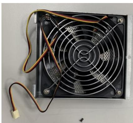
**Step 5** Screw the fan module to the system chassis and plug the fan cable to the fan connector on the riser.
