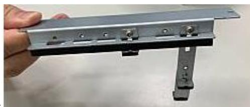
**Step 6** Fasten the holder bracket in the chassis, adjust the screw position of the extension bracket to fix the add-on card, and then tighten the screws.
