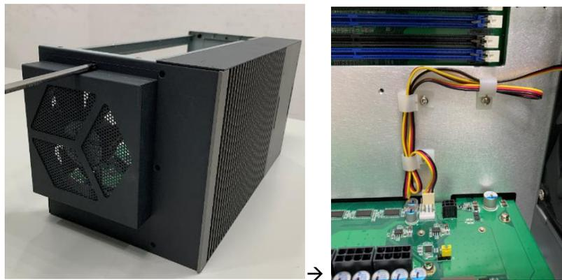
**Step 7** Close the side cover back to the chassis and fasten all screws. The installation is complete.
