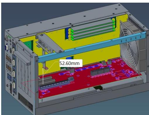
**Step 5** Connect the extension holder bracket to the holder bracket. The procedure is illustrated below.
