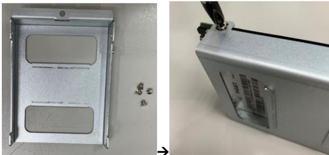
**Step 3** Align the connector of the SSD/HDD with the SATA slot (#1), then insert the SSD/HDD into the bay and screw the bracket. Installation is complete.
