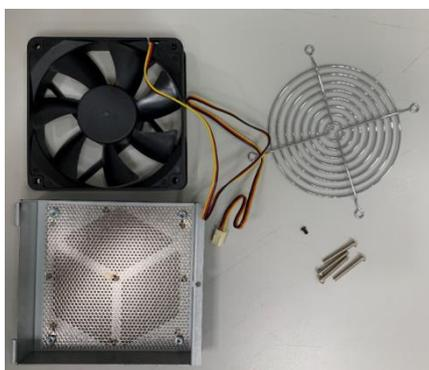
**Step 5** Put the fan on the fan bracket and screw the fan to the bracket.
