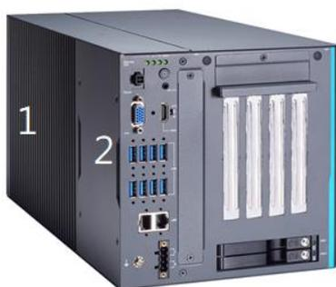
**Step 4** Insert the wireless LAN card into the mini card slot (1) or M.2 key socket (2) and push it down firmly. Then screw the card tightly to the mainboard.
