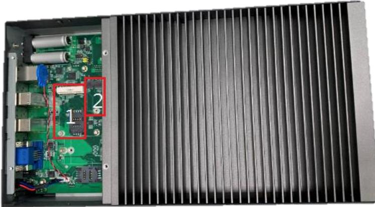
**Step 5** Remove the antenna plug from the front side, and then install the antenna on the antenna connector. The installation is complete.
