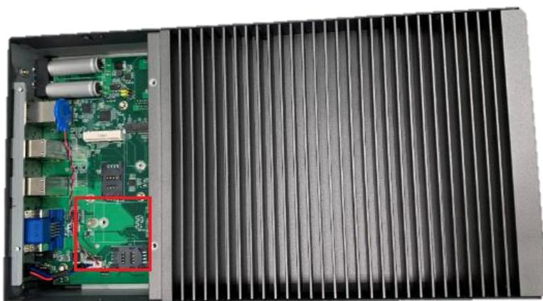
**Step 5** Remove the antenna plugs from the 5G bracket, install the antennas on the antenna connectors, and then screws the 5G bracket to the chassis. The installation is complete.
