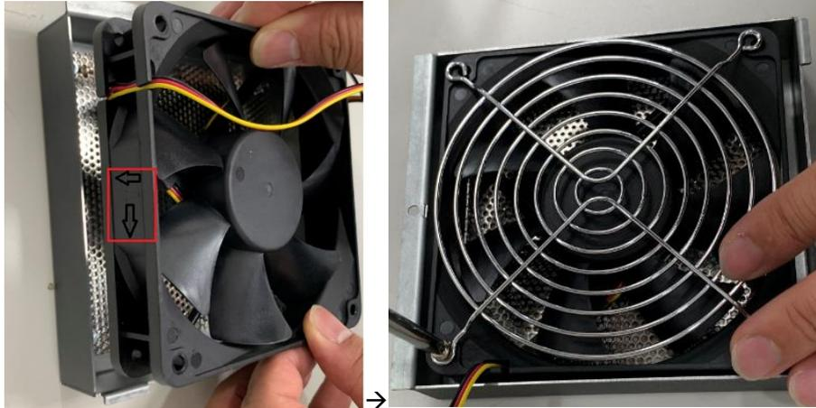
**Step 6** Screw the fan module to the system chassis and plug the fan cable to the fan connector on the riser.
