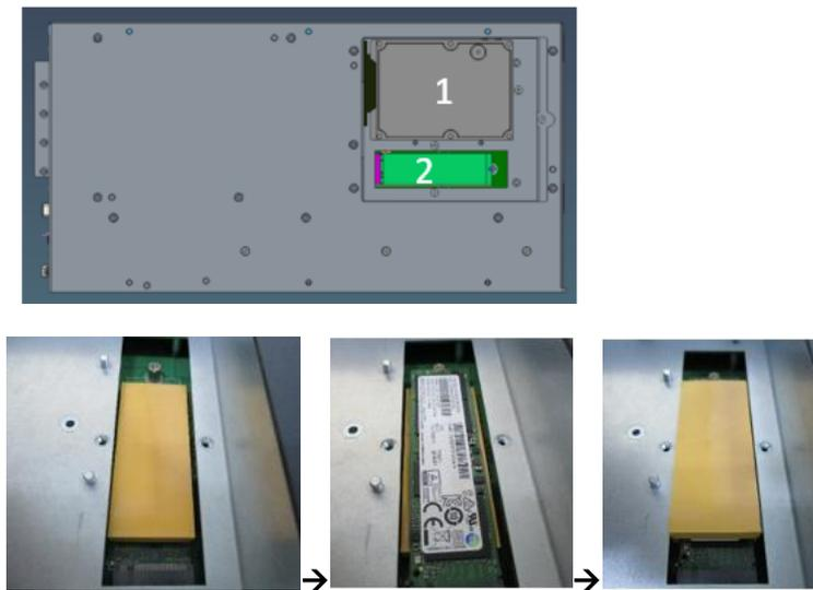
**Step 5** Screw the bracket with 2 screws. Installation is complete.
