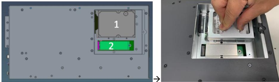
**Step 4** Take the NVMe bracket, thermal pads and its screws from the accessory box and stick a thermal pad on socket, then insert the SSD into the socket (#2) and screw it. Stick another pad on SSD.
