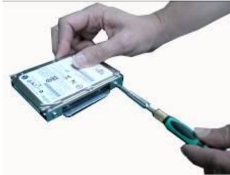
**Step 6** Install and fix the HDD through the side, next, plug the power cable in HDD.
