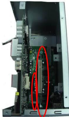
**Step 5** Align the PCI or PCIe card with the slot, and press the card into the slot until it is firmly seated.
