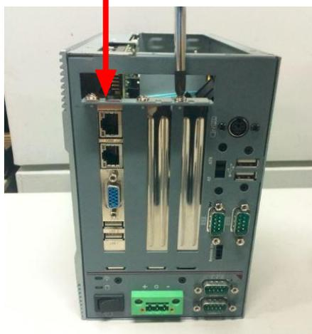
**Step 6** Close the top cover back to the chassis and fasten all screws.
