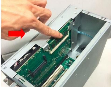
2. Install the memory module into the socket and push it firmly down until it is fully seated. The socket latches are clipped on to the edges of the SO-DIMM.
