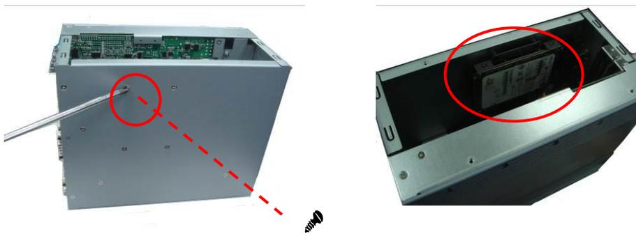
**Step 7** Close the top cover back to the chassis and fasten all screws.
