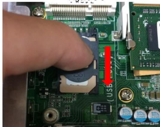
**Step4.** Insert the wireless module into the slot which marking with “USB/PCIe”.
