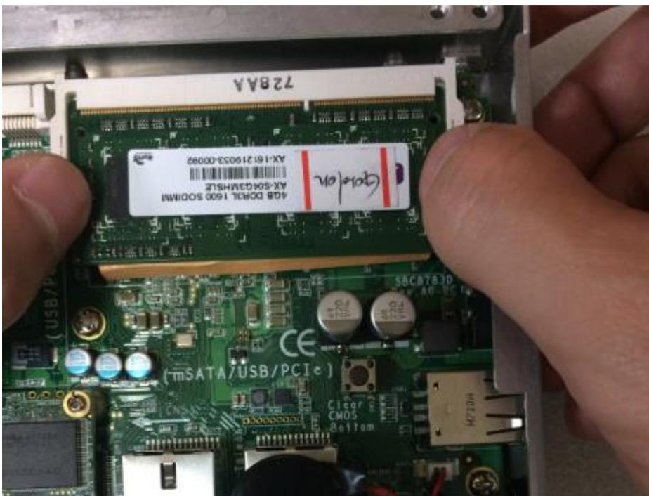
**Step 5** The memory module is locked by two latches on the sides. We strongly recommend using “LDC737” silicone on the two sides of the memory for good ability of vibration.
