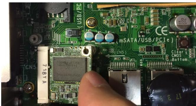
**Step 4** Fasten the screw tightly.
