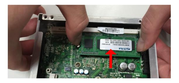
Step 4 The memory module is locked by two latches on the sides. We strongly recommend using "LDC737" silicone on the two sides of the memory for good ability of vibration.
