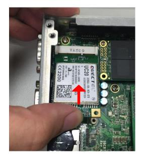
Step5. Insert the 3G module and screws it tight.
