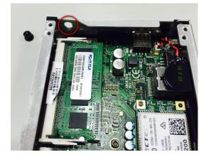
Step7. Connect the RF cable to the connector of 3G module which remarking "MAIN".
