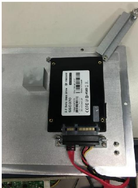
**Step 5** Screw the thumbscrew. Installation completed.
