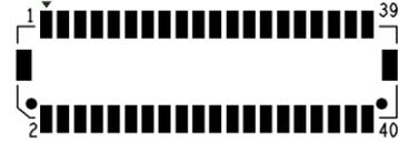
**HDD power connector: CN6**
