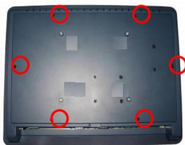
**Step 2** Find out the HDD slot in back cover.
