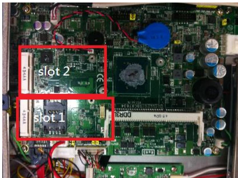
**Step 2** Insert the mSATA card to the slot 2. Screw it firmly on the slot.
