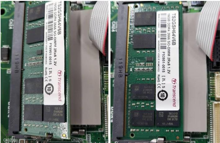
Figure 2-18: Installing a memory module
