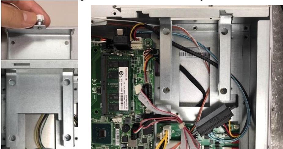
**Step 3** Insert the 2.5" HDD into the bracket and fasten the four screws on the bottom side of the bracket to hold the HDD firmly to the bracket.
