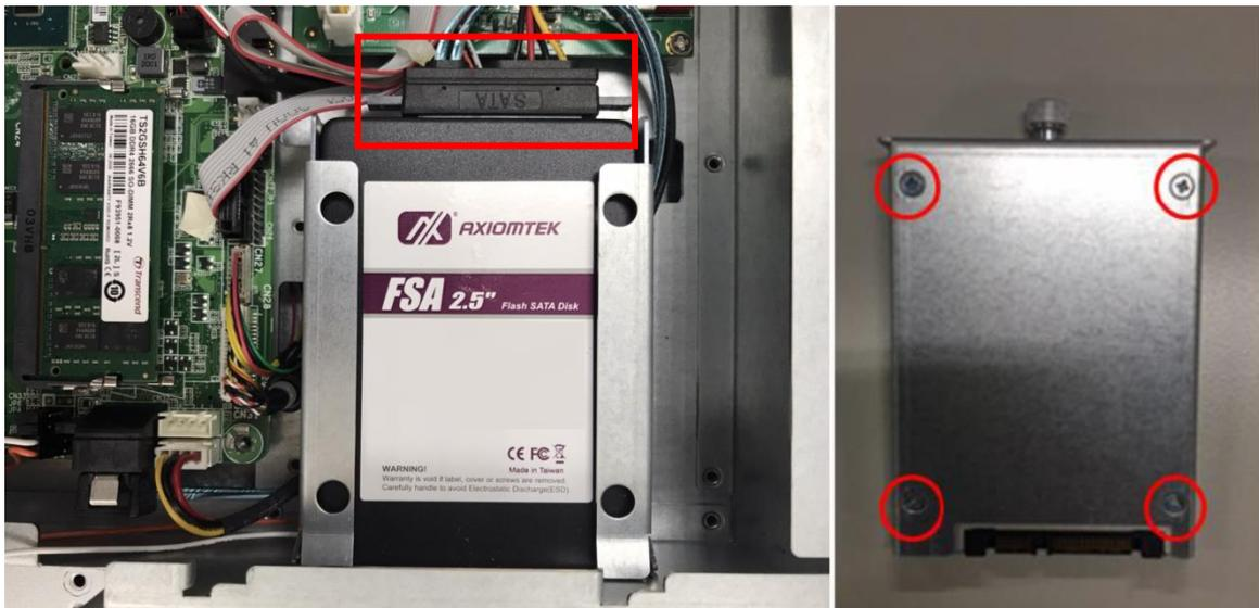
Figure 2-14: Fasten an HDD to the bracket and plug in the "SATA + Power" connector
