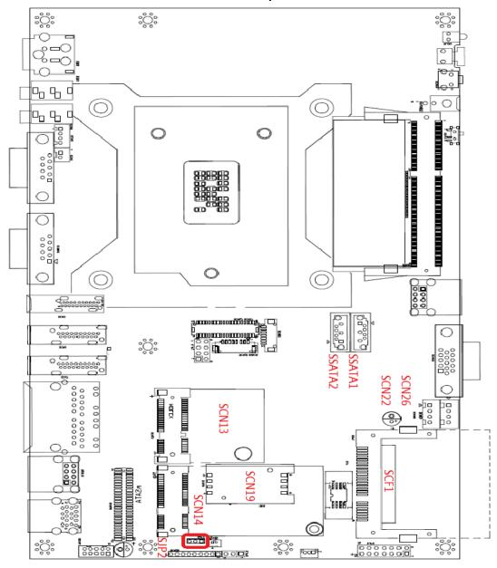
Jumper is a small component consisting of jumper clip and jumper pins. Install jumper clip on 2 jumper pins to close. And remove jumper clip from 2 jumper pins to open. The following illustration shows how to set up jumper.
