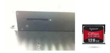
Step 3 Insert the CFast card to the CFast card slot, then finding the CFast cover and screw it.
