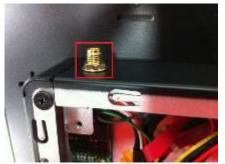
Remove the antenna plug from the top of back cover, and then install the Step 4 antenna on the antenna connector
