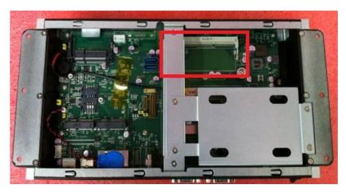
Step 3 Insert the DRAM to the DIMM socket, and then push it down firmly until it is clipped by the socket. Installation completed
