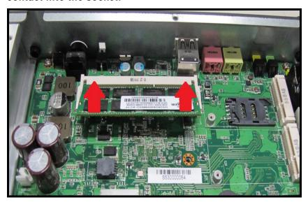
Step 6 Push the module down, until it is firmly seated by locking two latches on the sides.
