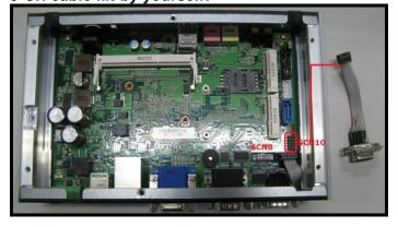
Step 5 Please notice the high spot of connector (10 pin) then connect it into SCN10. The high spot should be faced the mini card side.
