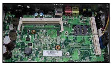
Step 4 Slide Mini PCIe Card into Mini PCIe slot with caution and fasten screw of Express Mini Card.
