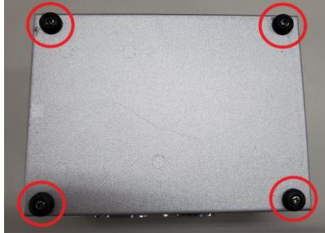
**Step 3** Open the bottom cover and Locate M.2 2230 key E connector within the red line as marked.
