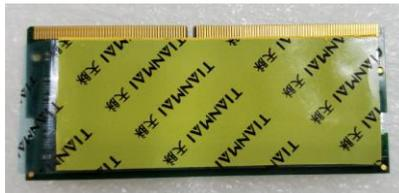
**Step 6** Insert a gold-colored contact into the socket and push the module two end latches till locked and then fasten the thermal pad bracket on top of the DRAM.
