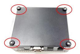
Step 3 Please find the HDD bracket location then loosen four screws of HDD bracket to take out it.
