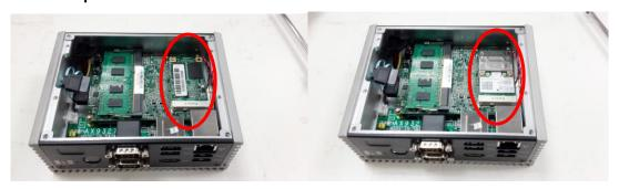
Step 6 Assembly the bottom cover back and fasten all screws.
