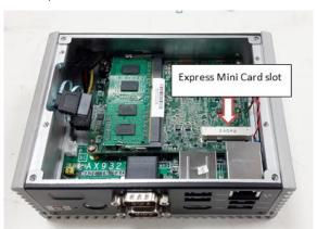
Step 5 Slide Mini Card into Mini Card slot with caution, and fasten screw of Express Mini Card.
