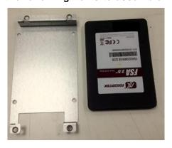
Step 6 Fasten total four screws to fix HDD/SSD.
