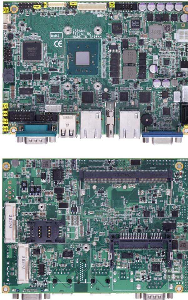
The CAPA841, a 3.5" board, supports Intel® Atom™ E3845/E3827 processors. Meanwhile CAPA842, a 3.5" board, supports Intel® Celeron® J1900/N2807 processors. Both of them deliver outstanding system performance through high-bandwidth interfaces, multiple I/O functions for interactive applications and various embedded computing solutions.
