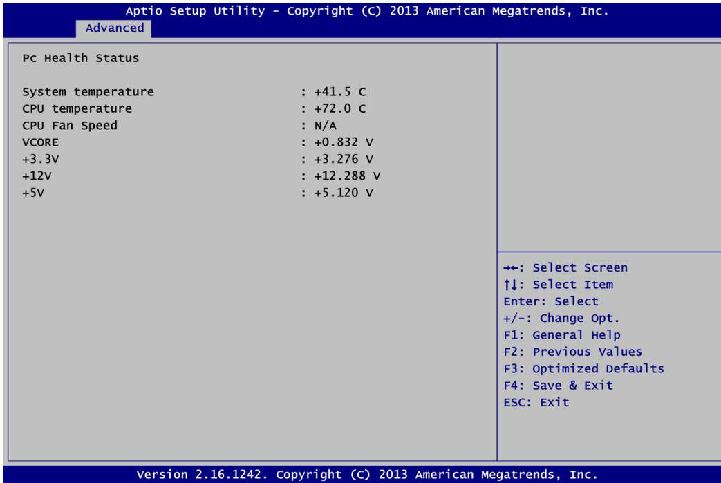
This screen displays the temperature of system and CPU, system voltages (VCORE, +3.3V, +12V and +5V).
