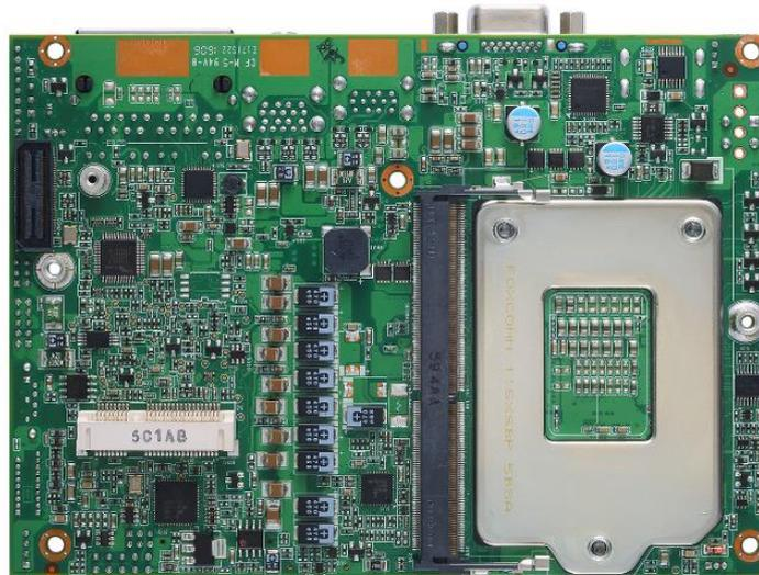
The CAPA500, a high performance 3.5" board, supports LGA1151 socket for 6<sup>th</sup>/ 7<sup>th</sup> Generation Intel® Core™ i7/ i5/ i3 processors with H110 (Q170 optional) chipsets. The board delivers outstanding system performance through high-bandwidth interfaces, multiple I/O functions for interactive applications and various embedded computing solutions.
