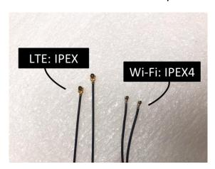
Step 7 Connect the SMA cables to the I-PEX connector of the wireless network Module and install antennas.
