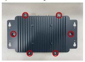
Step 3 After removing the bottom cover, locate the M.2 2242 Key B slot on the board, then take two thermal pads out of the package box, and apply one thermal pad on the M.2 2242 Key B slot-
