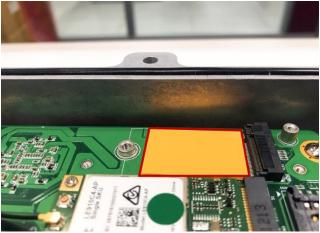
Step 4 While holding the M.2 2242 Key B SSD at a 30-degree angle up from the horizontal, slowly insert the golden finger into the M.2 2242 Key B slot until it is fully inserted in place. And secure the M.2 2242 Key B SSD to the carrier by tightening up one M3\*3L screw to the marked position. Then apply another thermal pad on the M.2 2242 Key B SSD.
