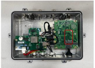
Step 4 While holding the PCI Express mini card at a 45-degree angle up from the horizontal, slowly insert the golden finger into the PCI Express slot until it is fully inserted in place.
