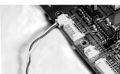
Photo 4 - Plug the soft switch bottom cable into the power connector of the Axiomtek backplane.
